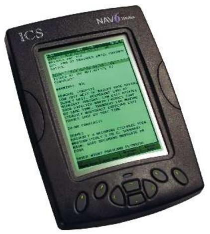
Figure 5 – Example of NAVTEX receiver with LCD screen
