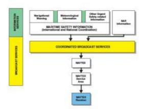
Figure 1 – Basic concept of the NAVTEX system
